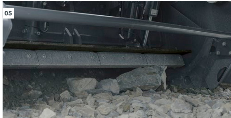
03 The carbide-edged crusher bars of the fixed and variable crushing stage act as counterblades that work in unison with the HT18 crushing tools and enable the rock to be crushed.
