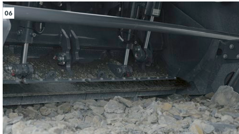
04 Coarse rocks build up in front of the active front door. 05 The active front door is opened manually and the material is pushed into the crushing and mixing housing as the machine advances. 06 The active front door is closed to minimize the ejection of material towards the front.
