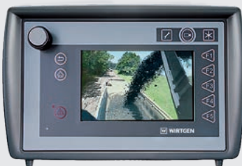
2 | Camera at end of conveyor
