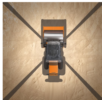
Unobstructed view backwards with no intrusive exhaust pipe. All models exceed the requirements of the standard for visibility.
