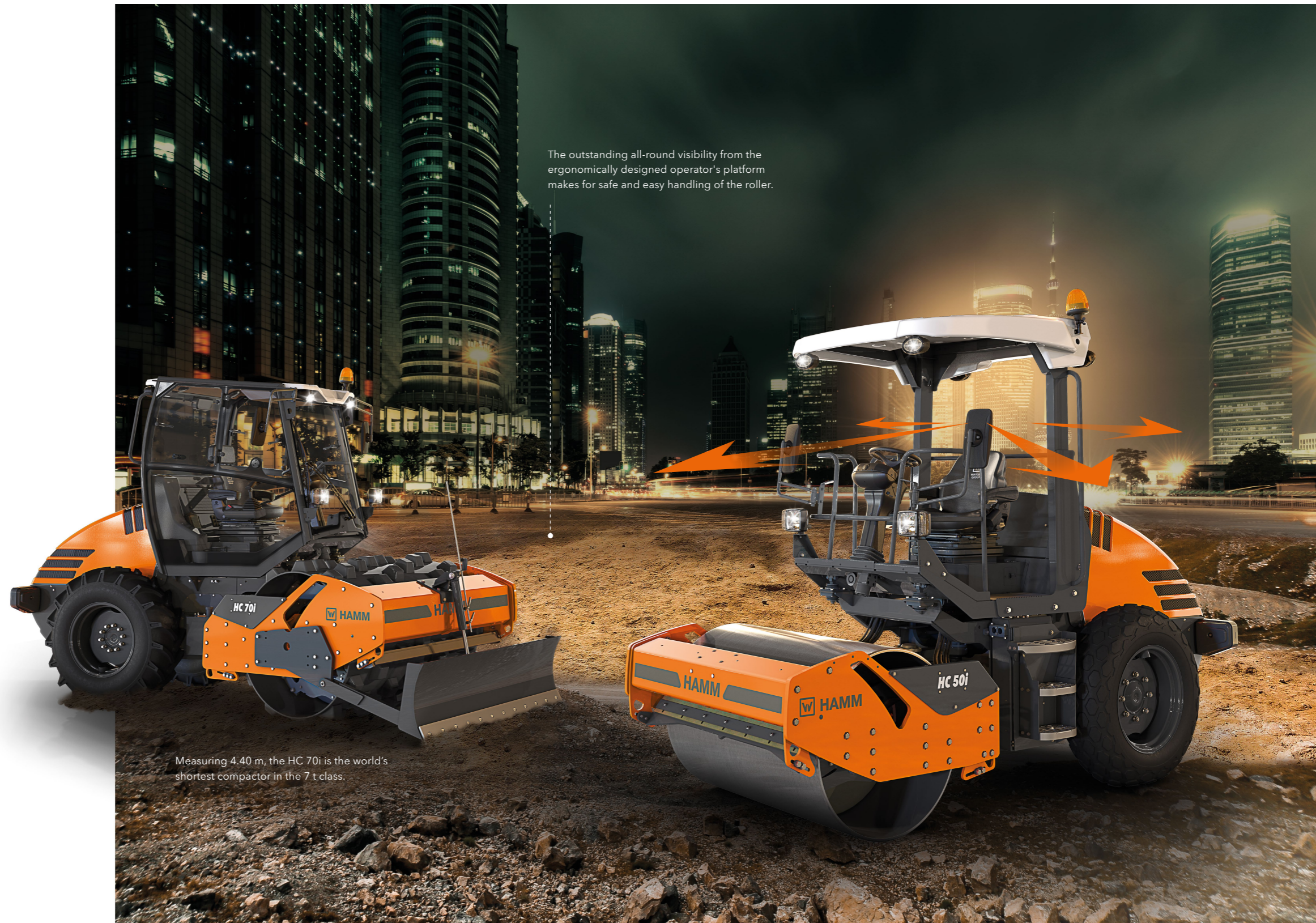
Unobstructed view backwards with no intrusive exhaust pipe. All models exceed the requirements of the standard for visibility.
