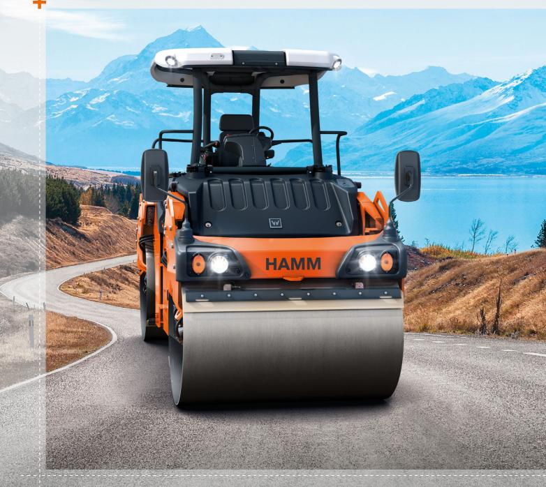
With over 50 models, the articulated tandem rollers in the HD+ series cover the range between 7 and 14 t. The XXL cabin or platform is very spacious and comfortable. From this ergonomically optimised workstation, drivers have an excellent overview of the drums, water-sprinkling system and surrounding area. The HD+ series offers impressive handling and compaction thanks to the 3-point articulation and homogeneous weight distribution.
