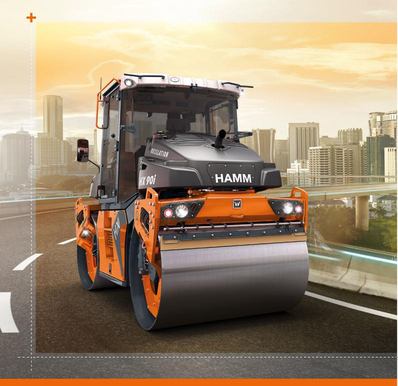
In the HX series tandem rollers, the Easy Drive operating concept provides top-class ergonomics and comfort. The fully glazed panoramic cabin or platform offers optimal visibility. Drivers have a good overview of the drum edges, the edge pressing and cutting device and the construction site at all times. Viewing panes in the cabin floor also allow an uninterrupted view of the drums or wheels. The HX series has pivot steering with very large track offset and large turning angles.
