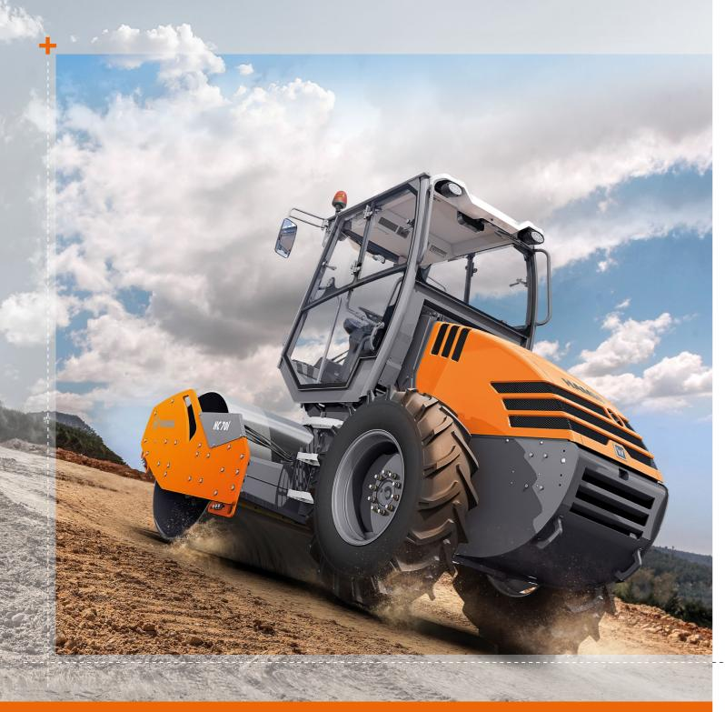
The extremely compact, very short compactors of the HC CompactLine series offer a huge gradeability of up to 60% and maximum ground clearance. They are driven by modern wheel motors. The very short wheelbase and 3-point articulation ensure optimal driving and handling characteristics - ideal for cramped construction sites and for compaction on rough terrain.
