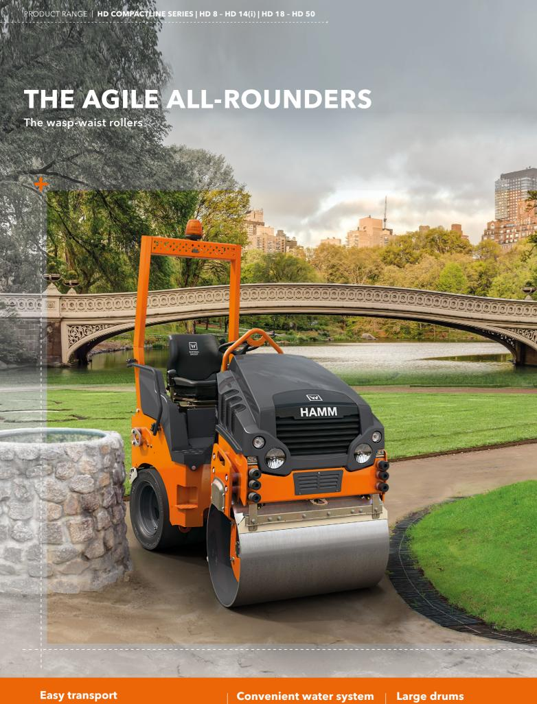
The articulated compact rollers in the HD CompactLine series are all-rounders for asphalt construction, earthworks and landscape gardening. Their operation is extremely easy and requires no special language skills. The wasp-waist design provides optimal visibility, and the 3-point articulation ensures outstanding driving and handling characteristics.
