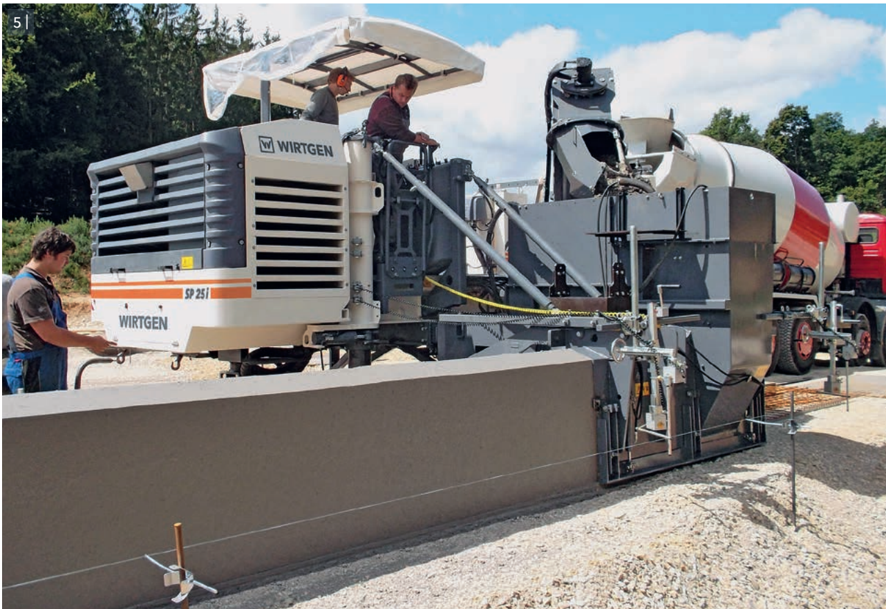
4-5 | The mold can be mounted on the left or right - modification is completed within an extremely short time.
