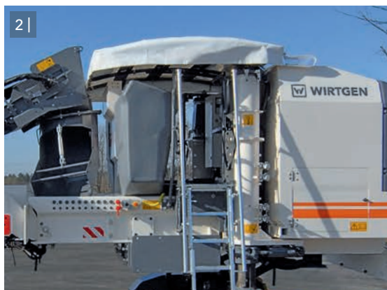
3 | In folding design, the belt conveyor can be folded hydraulically for transport.
