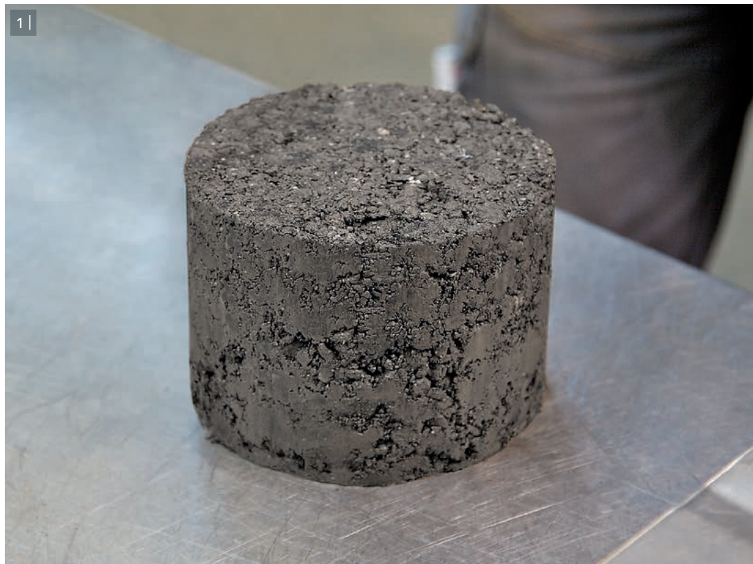
11 | Material treated with foamed bitumen impresses with high strength and bearing capacity.
