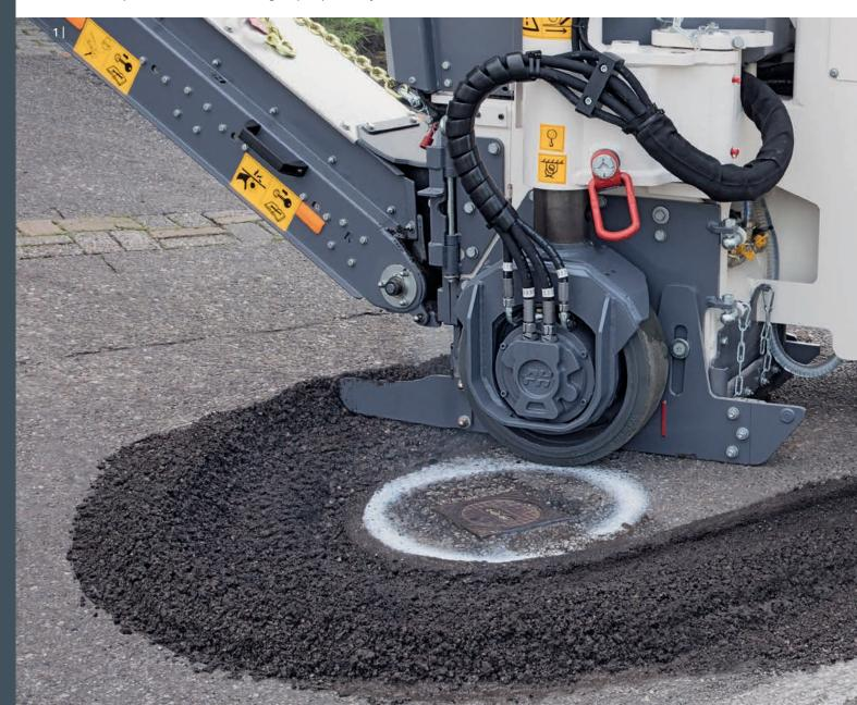
1 - 2 | The electronically controlled travel drive makes high-precision milling possible - such as around road installations, for example.
