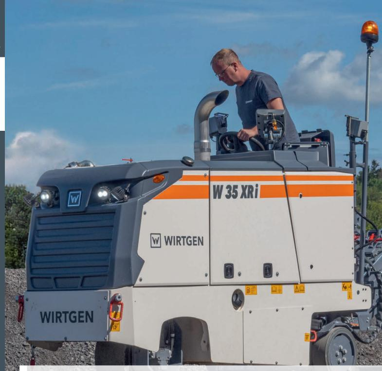
The highly maneuverable cold milling machine is perfect for milling jobs in confined spaces.
