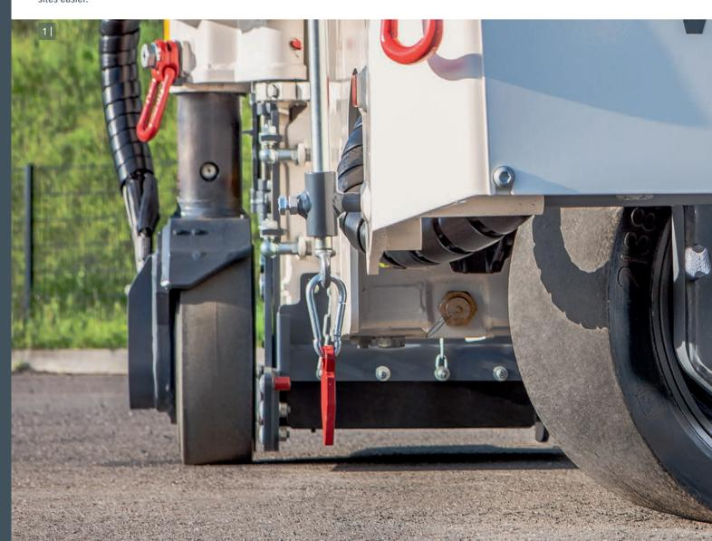
2 The small milling machine is ideally suited for fast maneuvering in narrow areas - also thanks to the ability to simply swing in the right rear wheel.
