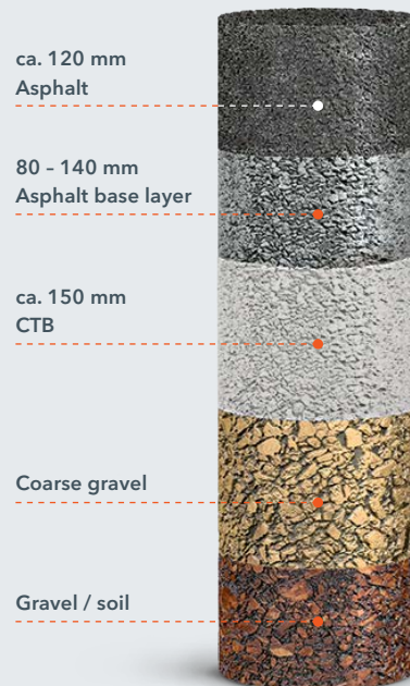
Road structure with CTB (example)
