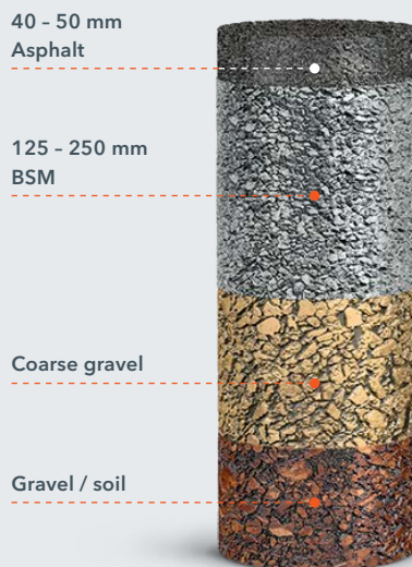
Road structure with BSM (example)
