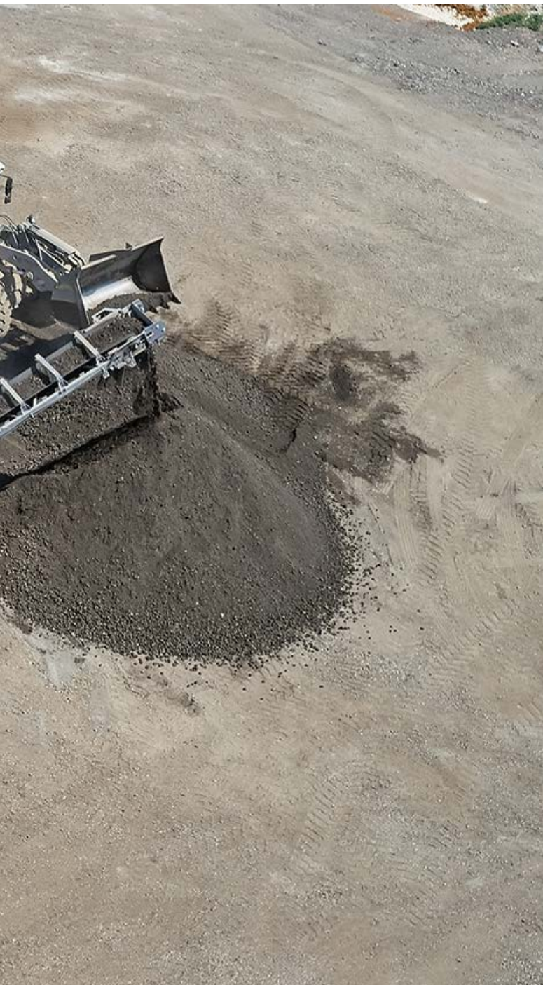
01 The mobile mixing plant is set up at the most logistically convenient location - including flexible, space-saving alignment. Here, storable mix is produced and stock-piled, then loaded onto trucks by a wheel loader.
