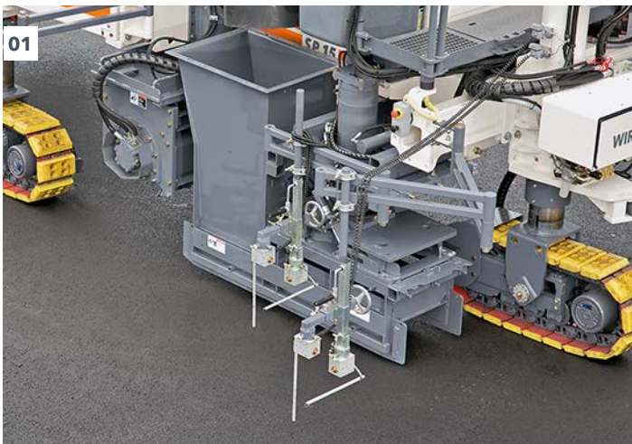
01 - 02 The mold can be telescoped outwards hydraulically by up to 700 mm.
