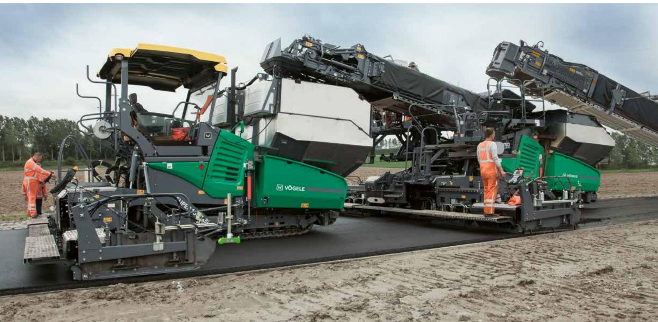
The extra conveyor unit is heated to prevent mix from sticking. For a safe clearance between pavers placing binder and surface course mixes, electronic distance control and an anti-collision protection are installed. For the storage of binder, an extra hopper holding 20 tonnes and insulated against loss of heat is available, to be placed into the paver’s material hopper.
