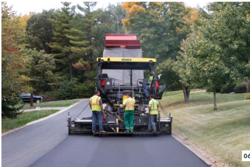
04 Significantly smaller turning radius due to Pivot Steer steering brake. 05 Optimum feeding with mix thanks to the large material hopper. 06 The right screed for every application. The paver can be combined with the VF 600, VR 600 and AB 600 Extending Screeds.
